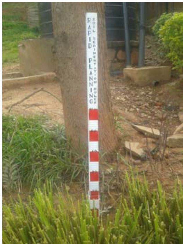
05/18 Soil Sedimentation Ruler installation, trapped ca. 20cm soil at 1 st line
